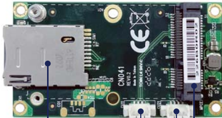
SIM Card Slot (Push-Push) (CU11~CU21) USB 2.0 PIN Header Mini PCIe Full-Size (USB only)
