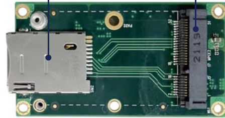
SIM Card Slot (Push-Push) (CU11~CU21) USB 2.0 PIN Header Mini PCIe Full-Size (USB only)
