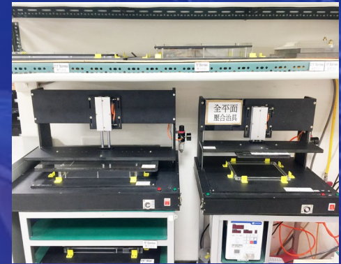
(Panel & Touch )Air leak & lamination test machine
